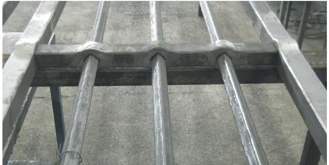
Detail of drilling in horizontal bars
