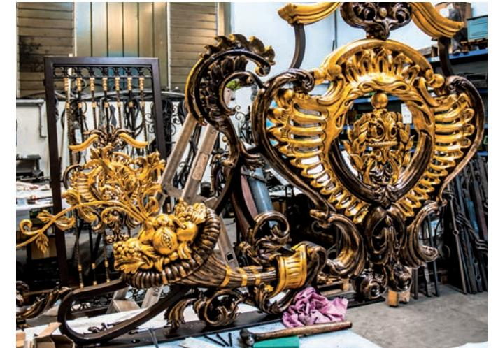
Detail of assembly of twisted bars and central decorations in polished brass protected with special paint
