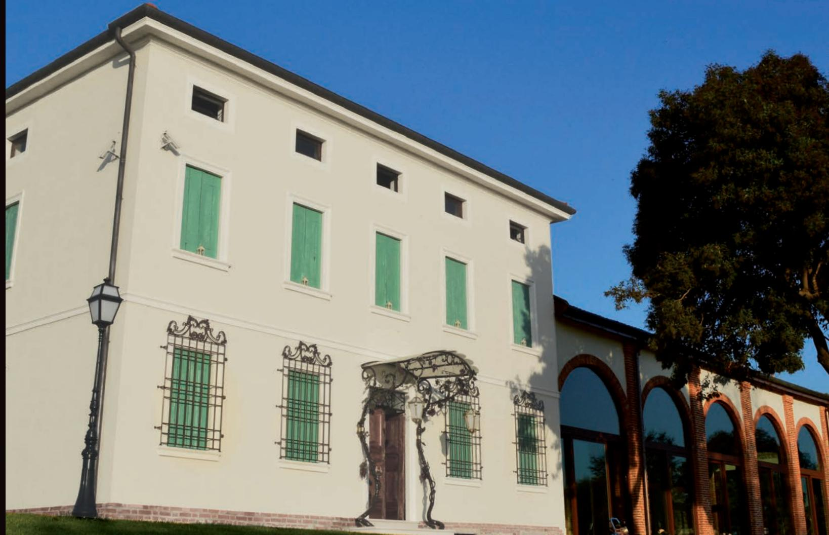
For this renowned Venetian farm, external elements were made consisting entirely of corten steel. This canopy at the entrance to the property deserved to be emphasised, so it was pre-forged by hand to simulate the natural sinuosity of a vineyard. Stainless steel railings were also made as part of the same project, which were then mirror polished around the intersections.
